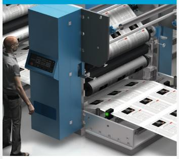
In printing presses, our USGT units are used to precisely align the paper for the upcoming printing. Here, the USGT excels with its high linearity and repeatability.
